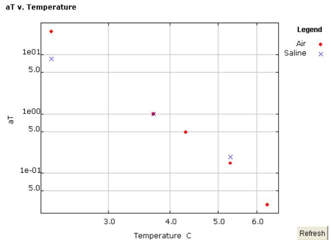
**Figure 5 Shift factors for master curve of UHMWPE**
