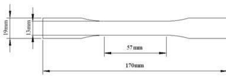
**Figure 3: ASTM D638 Type I test specimen geometry**
