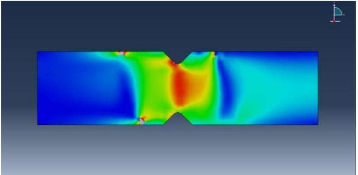
**Figure 9: Shear region at 0.2 mm crosshead displacement - Simulation**
