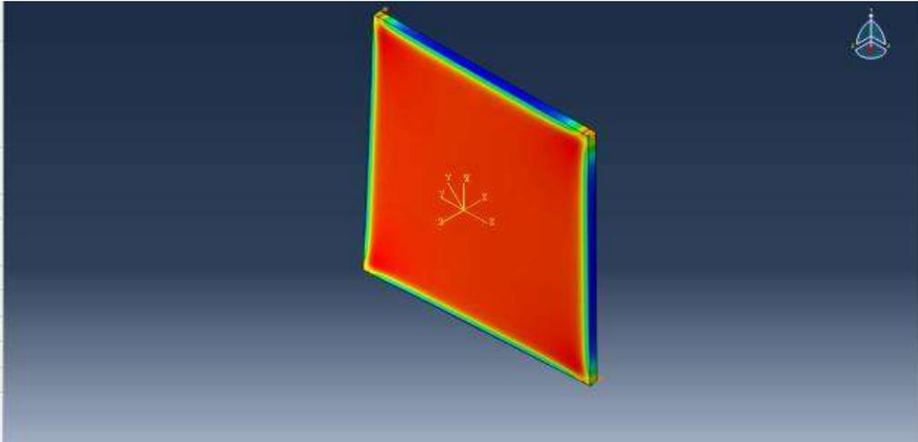
**Figure 12: Plate twist simulation showing shear region.**
