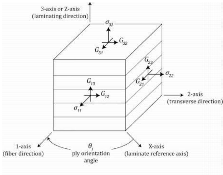
Figure 1: Composite coordinate system
