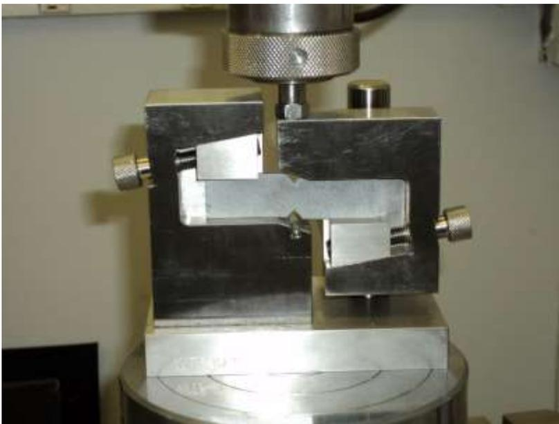
**Figure 5: Iosipescu shear fixture**
