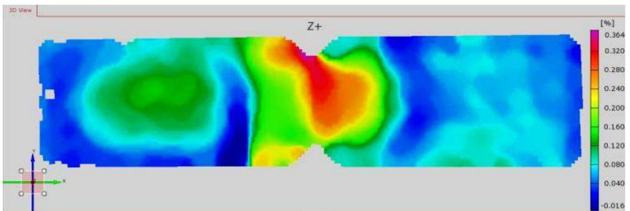
**Figure 10: DIC Image of the G12 measurement at 0.2mm displacement**
