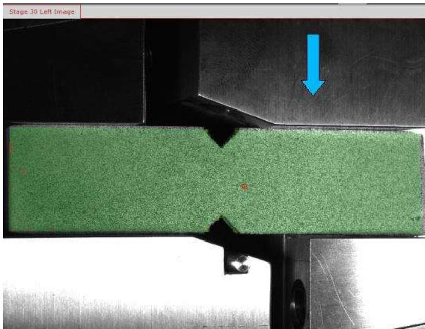
**Figure 6:** Speckle coated specimen in Iosipescu Fixture
