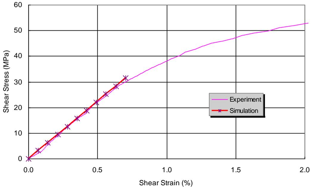
**Figure 11: Comparison of shear stress-strain G12 (simulation v. experiment)**
