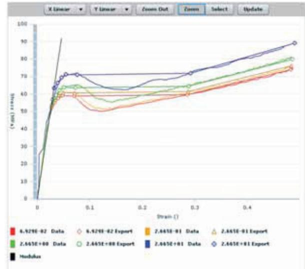
Figure 1: LS-DYNA MAT24 Crash Material Model Calibration
