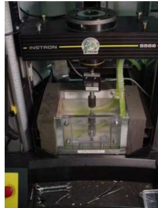
Mechanical stress-strain testing in a liquid, non-ambient environment
